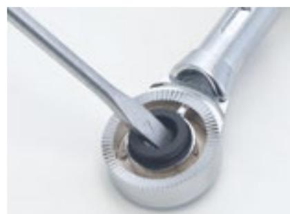
Easy and clever: Depending on the combination of your Basic Arm components simply remove a guide ring.
